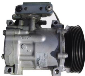
FIGURE 3-29 The decal on this compressor identifies the type (SDB709) and the serial number. Note also that it uses a seven-groove, multi-V clutch, four mounting bolts, and vertical-pad service ports at the side.
