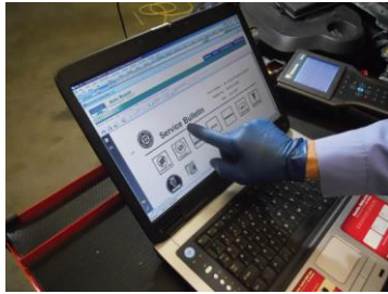
FIGURE 15-5 After checking for stored diagnostic trouble codes (DTCs), the wise technician checks service information for any technical service bulletins that may relate to the vehicle being serviced.
