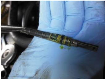
FIGURE 15–12 A partially restricted orifice tube should be replaced if discovered during service.
