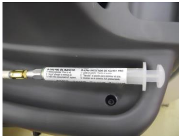
FIGURE 14–15 A variety of oil injectors are available for purchase. Some can be used while the system is under a vacuum, and some can force oil into a charged system.
