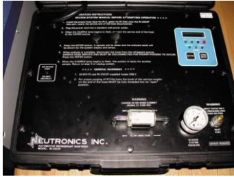
FIGURE 14-3 A typical refrigerant identification machine. The readout indicates what kind of refrigerant is in the system. If a blend or some other contaminated refrigerant is discovered, it should be recovered and stored in a separate container to keep it from contaminating fresh refrigerant.
