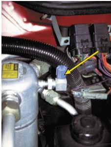
FIGURE 14-21 When a system is retrofitted from R-12 (CFC-12) to R-134a (HFC-134a), the proper service fittings have to be used to help assure that cross-contamination does not occur.
