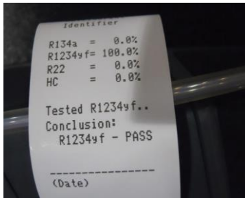
FIGURE 14-4 A typical printout showing that the system has 100% R-1234yf refrigerant in the system.
