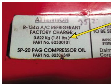
FIGURE 14-19 The underhood decal states that this vehicle requires 1.81 pounds (0.822 Kg) of R-134a refrigerant.
