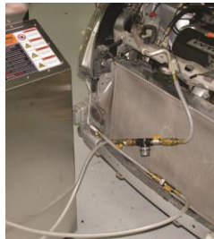
FIGURE 14-8 Portions of an A/C system can be flushed to remove debris and excess oil. Adapters are used to connect a flushing unit, which pumps the flushing material through the components. Most flushing machines are fully automated, meaning that it will vacuum, flush, recover, recycle, vacuum, and purge the cleaning solvent all automatically.
