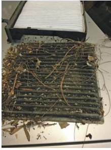
FIGURE 13-4 A dirty cabin filter removed from a Subaru that driver complained of poor cooling from the air conditioning system.
