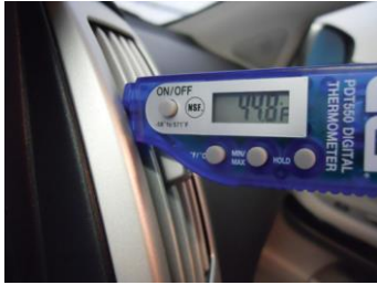
FIGURE 13-3 An air-conditioning thermometer being used to check the discharge temperature at the center vents.
