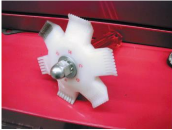
FIGURE 13-7 A fin comb is used to straighten the fins on the condenser to help increase airflow and heat transfer.
