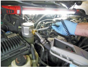
FIGURE 13-8 A typical electronic leak detector being used to locate a possible leak in a system.
