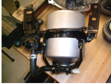
FIGURE 12-12 The storage tank and pump assembly as removed from underneath the vehicle. This pump is energized when coolant must be moved through the tank but the ICE is shut off.
