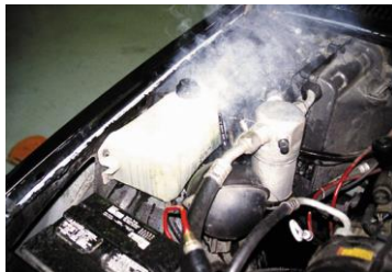
FIGURE 8-30 When an engine overheats, often the coolant overflow container boils.
