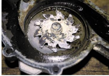
FIGURE 8-19 This severely corroded water pump could not circulate enough coolant to keep the engine cool. As a result, the engine overheated and blew a head gasket.
