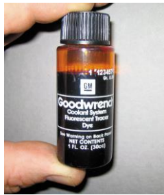
FIGURE 8-29 Use dye specifically made for coolant when checking for leaks using a black light.
