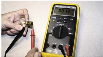
FIGURE 10-31 Using a digital multimeter set to read ohms ( \Omega ) to test this light bulb. The meter reads the resistance of the filament.
