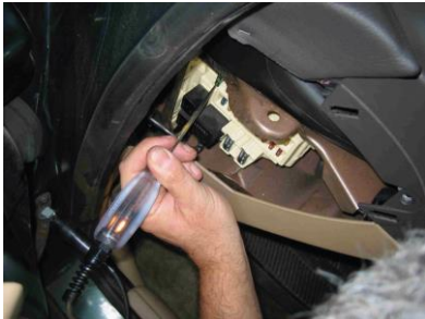
FIGURE 10–26 Testing a fuse with a test light. If the fuse is good, the test light should light on both sides (power side and load side) of the fuse.
