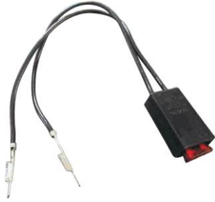
FIGURE 10–25 A technician-made fused jumper lead, which is equipped with a red 10-ampere fuse. This fused jumper wire uses terminals for testing circuits at a connector instead of alligator clips.
