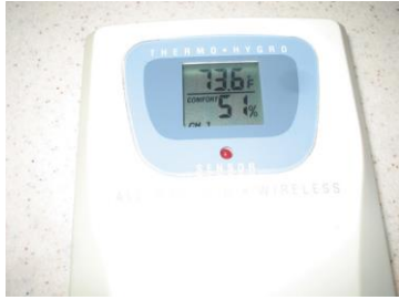
FIGURE 1-6 A combination meter that measures and displays both the temperature and the humidity is useful to use when working on air-conditioning systems.
