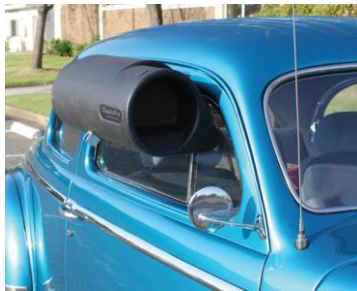
FIGURE 1-10 At one time, evaporative coolers were used to cool car interiors. Air forced through a water-wetted mesh produces evaporation and a cooling effect.
