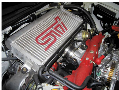
FIGURE 9-12 The unit on top of this Subaru that looks like a radiator is the intercooler, which cools the air after it has been compressed by the turbocharger.
