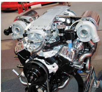
FIGURE 9-15 A dual turbocharger system installed on a small block Chevrolet V-8 engine.
