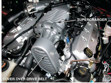
FIGURE 9-1 A supercharger on a Ford V-8.
