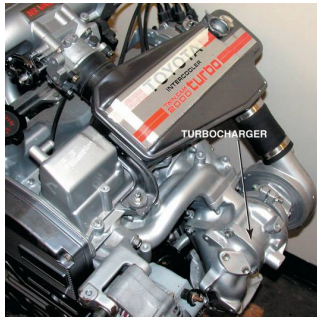
FIGURE 9-2 A turbocharger on a Toyota engine.
