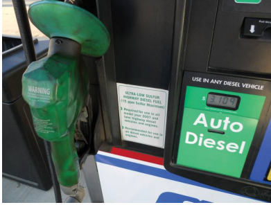
FIGURE 7-4 A pump decal indicating that the biodiesel fuel is ultra-low-sulfur diesel (ULSD) and must be used in 2007 and newer diesel vehicles.
