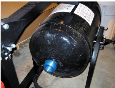
FIGURE 6-12 A CNG storage tank from a Honda Civic GX shown with the fixture used to support it while it is being removed or installed in the vehicle. Honda specifies that three technicians be used to remove or install the tank through the rear door of the vehicle due to the size and weight of the tank.
