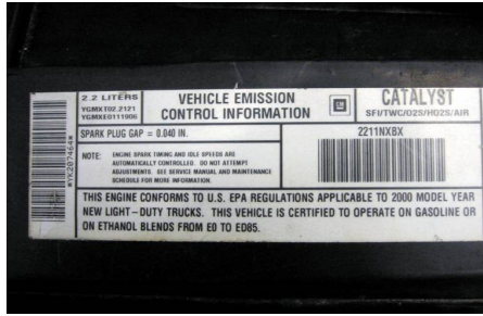
FIGURE 6-7 A vehicle emission control information (VEC) sticker on a flexible fuel vehicle indicating that it can use ethanol from 0 to 85%.
