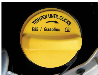
FIGURE 6-6 A flex-fuel vehicle often has a yellow gas cap, which is labeled E85/gasoline.
