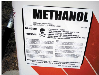
FIGURE 6-9 Sign on methanol pump shows that methyl alcohol is a poison and can cause skin irritation and other personal injury. Methanol is used in industry as well as being a fuel.
