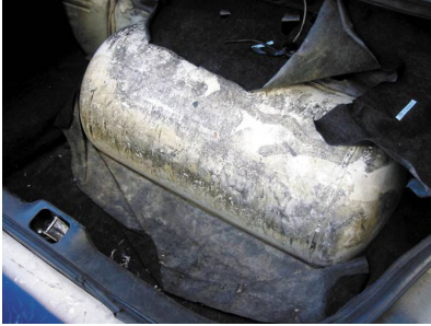
FIGURE 6-10 Propane fuel storage tank in the trunk of a Ford taxi.
