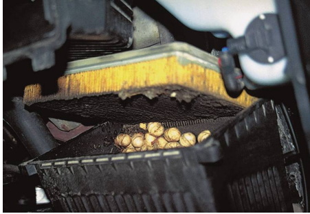
FIGURE 30-4 This is what was found when removing an air filter from a vehicle that had a lack-of-power concern. Obviously the nuts were deposited by squirrels or some other animal, blocking a lot of the airflow into the engine.
