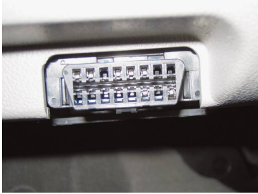
FIGURE 30-16 A typical OBD-II data link connector (DLC). The location varies with make and model and may even be covered, but a tool is not needed to gain access. Check service information for the exact location if needed.
