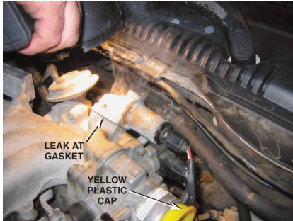
FIGURE 30-5 Using a bright light makes seeing where the smoke is coming from easier. In this case, smoke was added to the intake manifold with the inlet blocked with a yellow plastic cap and smoke was seen escaping past a gasket at the idle air control.
