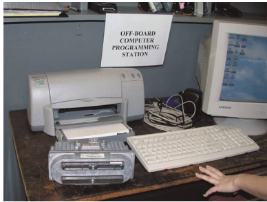
FIGURE 30-20 Connecting cables and a computer to perform off-board programming.
