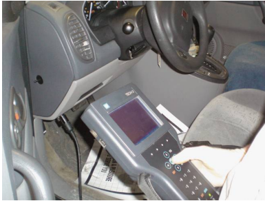
FIGURE 30-17 The first step in the reprogramming procedure is to determine the current software installed using a scan tool. Not all scan tools can be used. In most cases using the factory scan tool is needed for reprogramming unless the scan tool is equipped to handle reprogramming.
