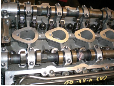
FIGURE 3-13 A DOHC engine uses a camshaft for the intake valves and a separate camshaft for the exhaust valves in each cylinder head.
