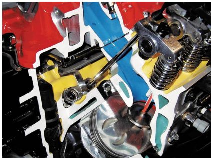
FIGURE 3-11 Cutaway of an overhead valve (OHV) V-8 engine showing the lifters, pushrods, roller rocker arms, and valves.
