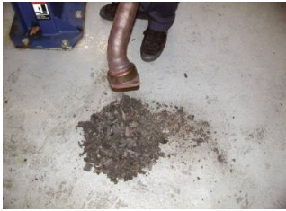
FIGURE 28-8 A catalytic converter that rattles when lapped was removed, and the substrate, or what was left of it, fell out. This converter has to be replaced and the root cause of why it failed found and corrected.
