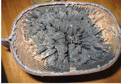
FIGURE 28-10 This partially melted catalytic converter tested okay at idle but had excessive back pressure at idle speeds.
