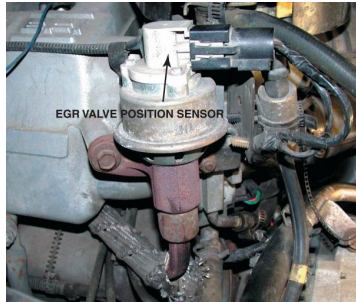
FIGURE 26-5 An EGR valve position sensor on top of an EGR valve.
