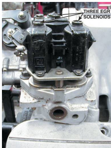
FIGURE 26-6 Digital EGR valve as used on some older General Motors engines.
