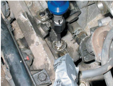
FIGURE 26-11 Removing the EGR passage plugs from the intake manifold on a Honda.
