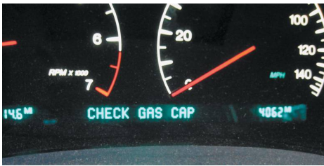
FIGURE 25-8 Some vehicles will display a message if an evaporative control system leak is detected that could be the result of a loose gas cap.
