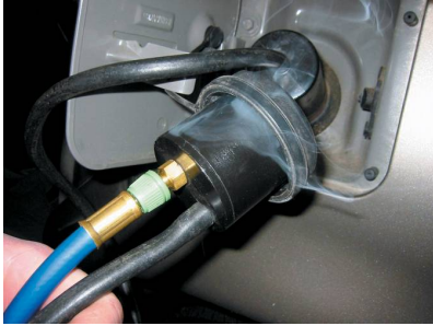
FIGURE 25-10 This unit is applying smoke to the fuel tank through an adapter, and the leak was easily found to be the gas cap seal.
