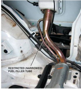
FIGURE 25-7 A restricted fuel fill pipe shown on vehicle with the interior removed.
