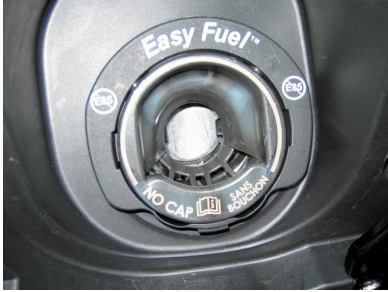
FIGURE 25-1 A capless system from a Ford Flex does not use a replaceable cap; instead, it is spring-loaded closed.
