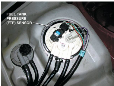
FIGURE 25-12 The fuel tank pressure sensor (black unit with three wires) looks like a MAP sensor and is usually located on top of the fuel pump module (white unit).
