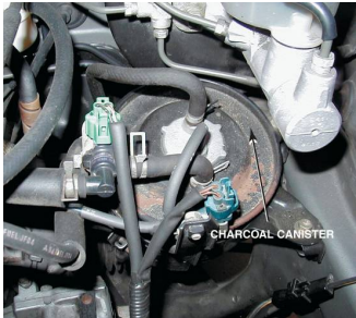
FIGURE 25-2 A charcoal canister can be located under the hood or underneath the vehicle.
