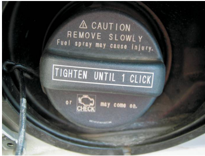
FIGURE 25-14 This Toyota cap warns that the check engine light will come on if not tightened until one click.
