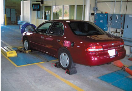
FIGURE 24-4 A vehicle being tested during an enhanced emission test.
