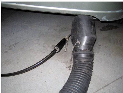
FIGURE 24-6 A partial stream sampling exhaust probe being used to measure exhaust gases in parts per million (PPM) or percent (%).
