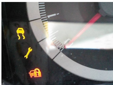
FIGURE 22-9 A wrench symbol warning lamp on a Ford vehicle. The symbol can also be green.
