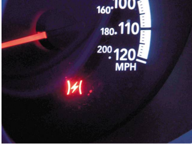
FIGURE 22-10 A symbol used on a Chrysler vehicle indicating a fault with the electronic throttle control.
