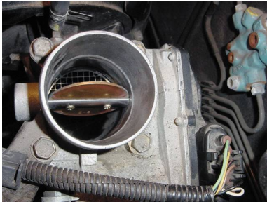
FIGURE 22-11 The throttle plate stayed where it was moved, which indicates that there is a problem with the electronic throttle body control assembly.
