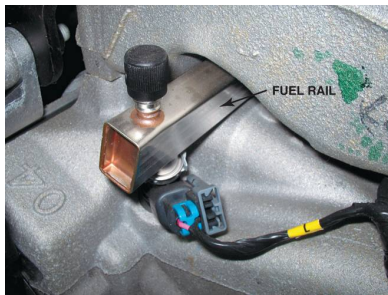
FIGURE 20-15 A rectangular-shaped fuel rail is used to help dampen fuel system pulsations and noise caused by the injectors opening and closing.
