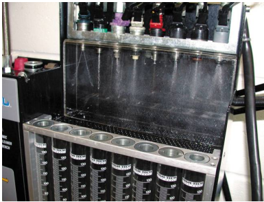
FIGURE 20-17 Each of the eight injectors shown are producing a correct spray pattern for the applications. While all throttle-body injectors spray a conical pattern, most port fuel injections do not.
