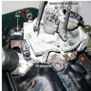
FIGURE 20-2 A dual-nozzle TBI unit on a Chevrolet 4.3-L V-6 engine. The fuel is squirted above the throttle plate where the fuel mixes with air before entering the intake manifold.
