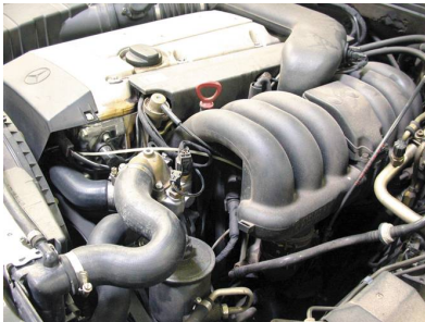
FIGURE 20-8 A port fuel-injected engine that is equipped with long, tuned intake manifold runners.
