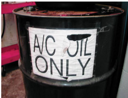
FIGURE 2-9 Air-conditioning refrigerant oil must be kept separated from other oils because it contains traces of refrigerant and must be treated as hazardous waste.
