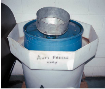
FIGURE 2-7 Used antifreeze coolant should be kept separate and stored in a leakproof container until it can be recycled or disposed of according to federal, state, and local laws. Note that the storage barrel is placed inside another container to catch any coolant that may spill out of the inside barrel.
