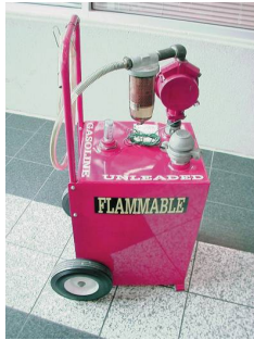
FIGURE 2-8 This red gasoline container holds about 30 gallons of gasoline and is used to fill vehicles used for training.
