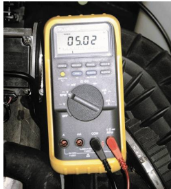
FIGURE 14-5 Checking the 5-volt reference from the computer being applied to the TP sensor with the ignition switch on (engine off).
