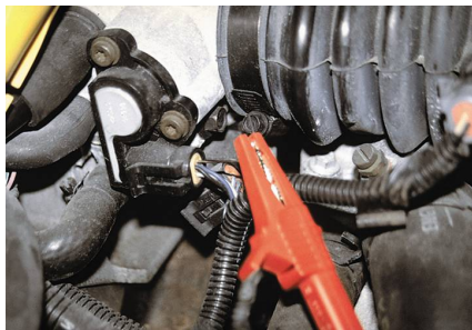
FIGURE 14-3 A meter lead connected to a T-pin that was gently pushed along the signal wire of the TP sensor until the point of the pin touched the metal terminal inside the plastic connector.
