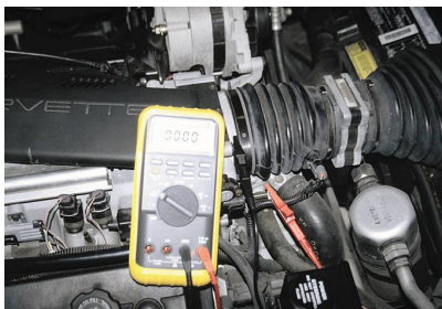
FIGURE 14-6 Checking the voltage drop between the TP sensor ground and a good engine ground with the ignition on (engine off). A reading of greater than 0.2 volt (200 mV) represents a bad computer ground.
