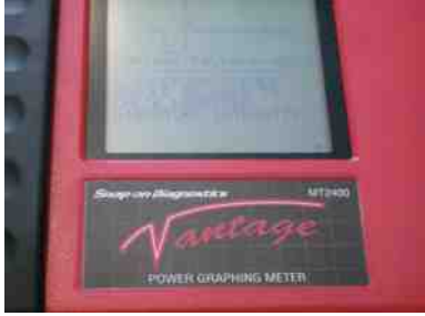
FIGURE 9-10 A typical graphing multimeter that can be used as a digital meter, plus it can display the voltage levels on the display screen.
