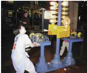
FIGURE 3-20 A display at the Henry Ford Museum in Dearborn, Michigan, that includes a hand-cranked generator and a series of light bulbs. This figure shows a young man attempting to light as many bulbs as possible. The crank gets harder to turn as more bulbs light because it requires more power to produce the necessary watts of electricity.
