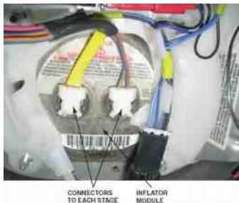
FIGURE 27-12 A driver's side airbag showing two inflator connectors. One is for the lower force inflator and the other is for the higher force inflator. Either can be ignited or both at the same time if the deceleration sensor detects a severe impact.
