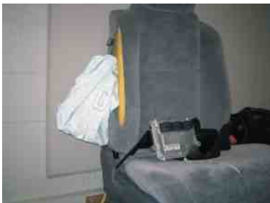
FIGURE 27-24 A typical seat (side) airbag that deploys from the side of the seat.
