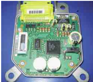
FIGURE 27-11 A sensing and diagnostic module that includes an accelerometer.
