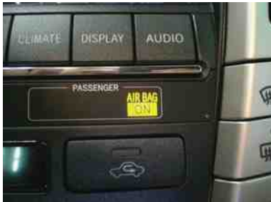
FIGURE 27-20 The passenger side airbag "on" lamp will light if a passenger is detected on the passenger seat.
