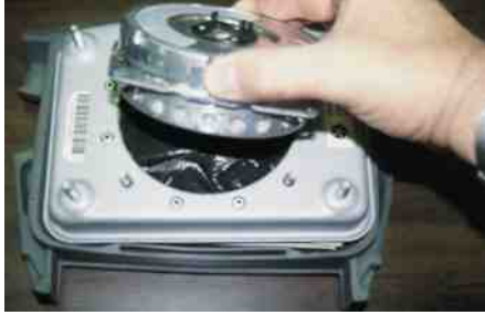
FIGURE 27-7 The inflator module is being removed from the airbag housing. The squib is the heating element that ignites the pyrotechnic gas generator that rapidly produces nitrogen gas to fill the airbag.
