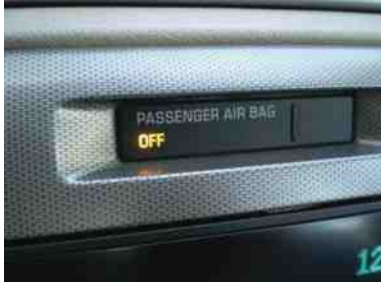
FIGURE 27-19 A dash warning lamp will light if the passenger side airbag is off because no passenger was detected by the seat sensor.
