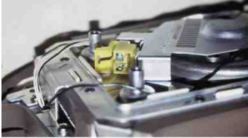
FIGURE 27-16 Shorting bars are used in most airbag connectors. These spring-loaded clips short across both terminals of an airbag connector when it is disconnected to help prevent accidental deployment of the airbag. If electrical power was applied to the terminals, the shorting bars would simply provide a low-resistance path to the other terminal and not allow current to flow past the connector. The mating part of the connector has a tapered piece that spreads apart the shorting bars when the connector is reconnected.
