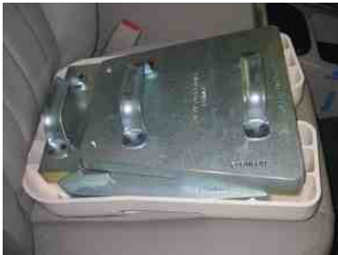
FIGURE 27-23 A test weight is used to calibrate the occupant detection system on a Chrysler vehicle.
