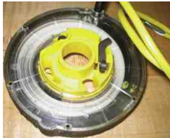
FIGURE 27-17 An airbag clockspring showing the flat conductor wire. It must be properly positioned to ensure proper operation.
