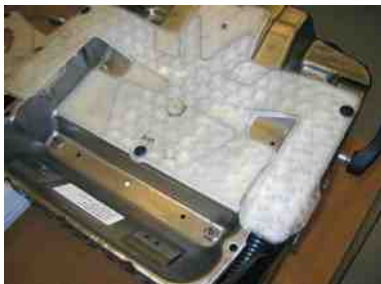
FIGURE 27-21 A gel-filled (bladder-type) occupant detection sensor showing the pressure sensor and wiring.
