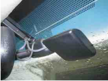
FIGURE 25-16 A typical rain sensing module located on the inside of the windshield near the inside rearview mirror.
