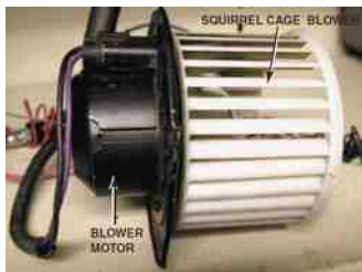
FIGURE 25-18 A squirrel cage blower motor. A replacement blower motor usually does not come equipped with the squirrel cage blower, so it has to be switched from the old motor.
