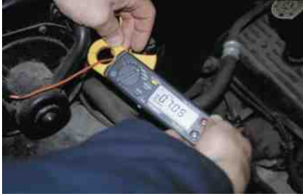
FIGURE 25-22 Using a mini AC/DC clamp-on multimeter to measure the current draw of a blower motor.
