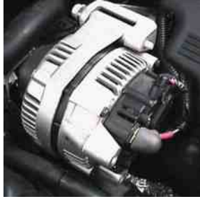
FIGURE 21-1 A typical alternator on a Chevrolet V-8 engine.
