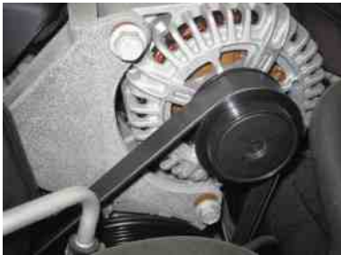
FIGURE 21-3 An OAP on a Chevrolet Corvette alternator.
