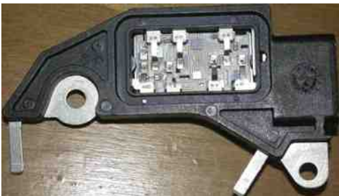
FIGURE 21-18 A typical electronic voltage regulator with the cover removed showing the circuits inside.
