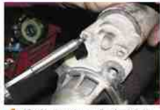
4 A Torx driver is used to remove the solenoid attaching screws.
