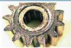
12 A close-up of one of the planetary gears, which shows the small needle bearings on the inside.
