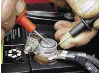
FIGURE 20-4 To test the voltage drop of the battery cable connection, place one voltmeter lead on the battery terminal and the other voltmeter lead on the cable end and crank the engine. The voltmeter will read the difference in voltage between the two leads, which should not exceed 0.20 volt (200 mV).
