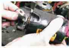
8 The structure assembly is removed from the field frame.
