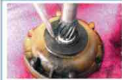
13 The lip is removed from the shaft so the planetary gear assembly can be separated and inspected.
