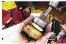
10 A light tap with a hammer dislodges the armature. Do not hit the jaws of the hands from the center of the gear reduction assembly.
