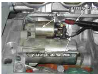
FIGURE 20-6 The starter is located under the intake manifold on this Cadillac Northstar engine.
