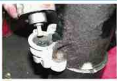
5 After the retaining screws have been reinserted, the solenoid can be separated from the starter motor. This retainer always replaces the solenoid.
