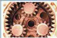
11 This figure shows the planetary ring gear and planet gears.
