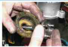
14 The shaft assembly is being separated from the stationary gear assembly.
