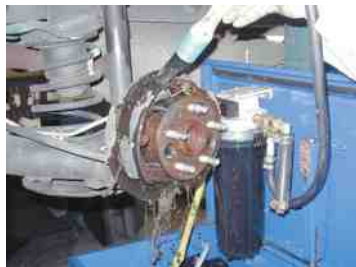
FIGURE 2-2 All brakes should be moistened with water or solvent to help prevent brake dust from becoming airborne.
