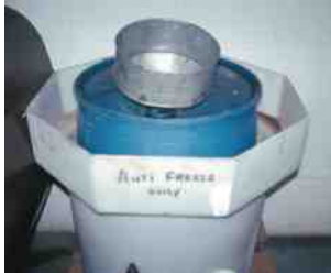
FIGURE 2-7 Used antifreeze coolant should be kept separate and stored in a leakproof container until it can be recycled or disposed of according to federal, state, and local laws. Note that the storage barrel is placed inside another container to catch any coolant that may spill out of the inside barrel.
