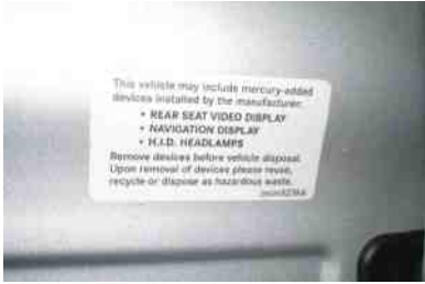
FIGURE 2-10 Placard near driver's door, including what devices in the vehicle contain mercury.
