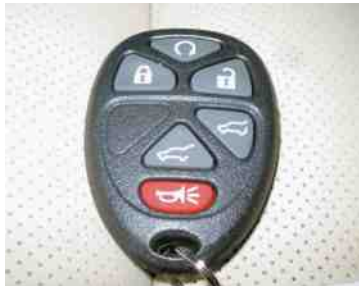
FIGURE 19-5 The top button on this key fob is the remote start button.
