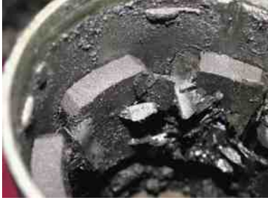
FIGURE 19-19 This starter permanent magnet field housing was ruined when someone used a hammer on the field housing in an attempt to "fix" a starter that would not work. A total replacement is the only solution in this case.
