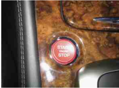
FIGURE 19-4 Instead of using an ignition key to start the engine, some vehicles are using a start button which is also used to stop the engine, as shown on this Jaguar.
