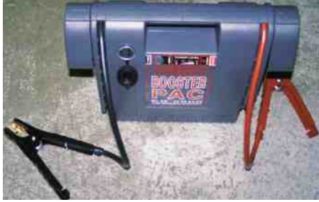
FIGURE 18-13 A typical battery jump box used to jump start vehicles. These hand-portable units have almost made jumper cables obsolete.
