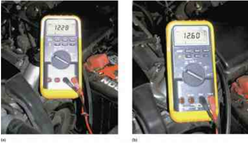
FIGURE 18-4 (a) A battery voltage of 12.28 volts is definitely not fully charged and should be charged before testing. (b) A battery that measures 12.6 volts or higher after the surface charge has been removed is 100% charged.
