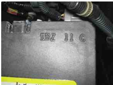
FIGURE 18-15 The code on the Delphi battery indicates that it was built in 2005 (5), in February (B), on the eleventh day (11), during third shift (C), and in the Canadian plant (Z).
