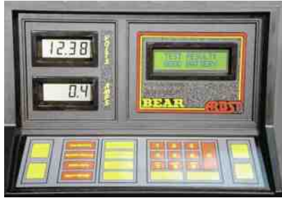
FIGURE 18-7 An alternator regulator battery starter tester (ARBST) automatically loads the battery with a fixed load for 15 sec. to remove the surface charge, then removes the load for 30 sec. to allow the battery to recover, and then reapplies the load for another 15 sec. The results of the test are then displayed.
