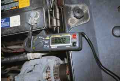
FIGURE 18-16 This mini clamp-on digital multimeter is being used to measure the amount of battery electrical drain that is present. In this case, a reading of 20 mA (displayed on the meter as 00.02 A) is within the normal range of 20 to 30 mA. Be sure to clamp around all of the positive battery cable or all of the negative battery cable, whichever is easiest to get the clamp around.
