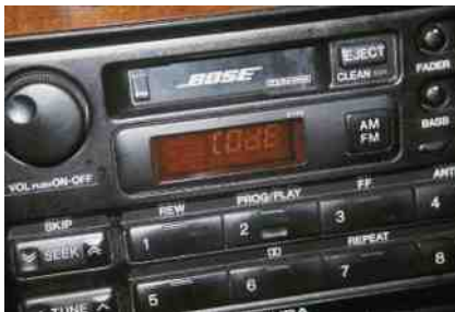
FIGURE 18-18 The battery was replaced in this Acura and the radio displayed “code” when the replacement battery was installed. Thankfully, the owner had the five-digit code required to unlock the radio.
