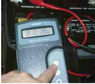
FIGURE 18-10 A conductance tester is very easy to use and has proved to accurately determine battery condition if the connections are properly made. Follow the instructions on the display exactly for best results.
