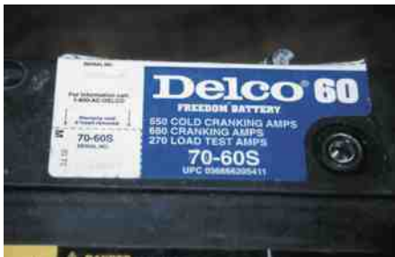
FIGURE 18-6 This battery has cold-cranking amperes (CCA) of 550 A, cranking amperes (CA) of 680 A, and load test amperes of 270 A listed on the top label. Not all batteries have this complete information.
