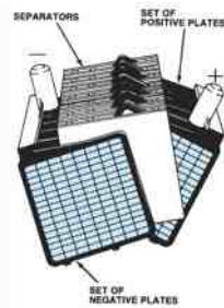
FIGURE 17-3 Two groups of plates are combined to form a battery element.
