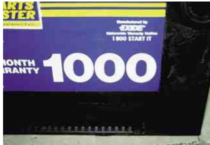
FIGURE 17-11 This battery has a cranking amperes (CA) rating of 1,000. This means that this battery is capable of cranking an engine for 30 seconds at a temperature of 32°F (0°C) at a minimum of 1.2 volts per cell (7.2 volts for a 12-volt battery).
