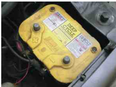
FIGURE 17-9 An absorbed glass mat battery is totally sealed and is more vibration resistant than conventional lead-acid batteries.
