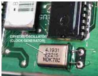
FIGURE 15-6 The clock generator produces a series of pulses that are used by the microprocessor and other components to stay in step with each other at a steady rate.
