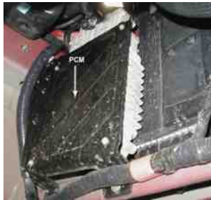
FIGURE 15-8 This PCM on a Chrysler vehicle can only be seen by hoisting the vehicle, because it is located next to the radiator and in the airflow to help keep it cool.
