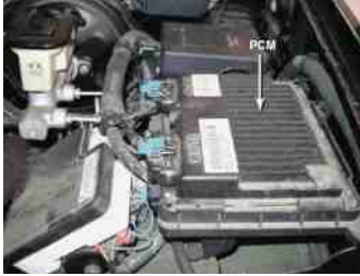
FIGURE 15-7 This powertrain control module (PCM) is located under the hood on this Chevrolet pickup truck.
