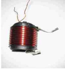
FIGURE 13-22 The coil-on-plug (COP) design typically uses a bobbin-type coil.
