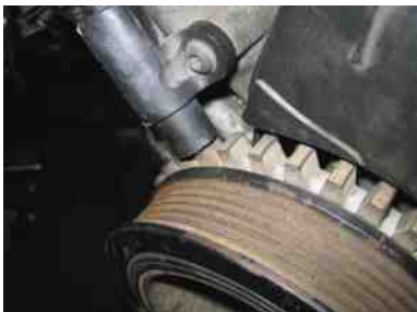
FIGURE 13-6 A crankshaft position sensor and reluctor (notched wheel).
