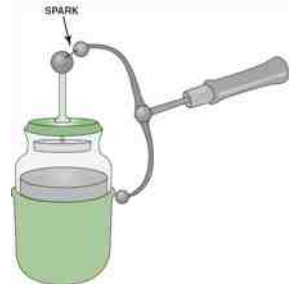
FIGURE 12-1 A Leyden jar can be used to store an electrical charge.
