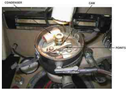
FIGURE 12-7 A point-type distributor shown with the condenser from an old vehicle being tested on a distributor machine.
