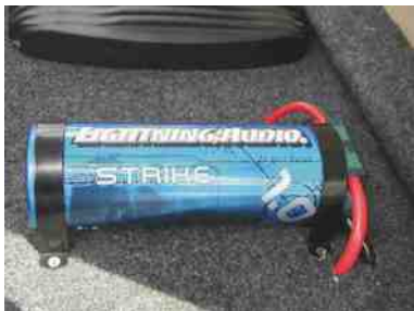
FIGURE 12-9 A 1 farad capacitor used to boost the power to large speakers.
