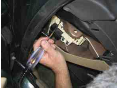
FIGURE 10-7 To test a fuse, use a test light to check for power at the power side of the fuse. The ignition switch and lights may have to be on before some fuses receive power. If the fuse is good, the test light should light on both sides (power side and load side) of the fuse.
