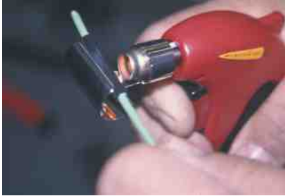
FIGURE 10-22 A butane torch especially designed for use on heat shrink applies heat without an open flame, which could cause damage.
