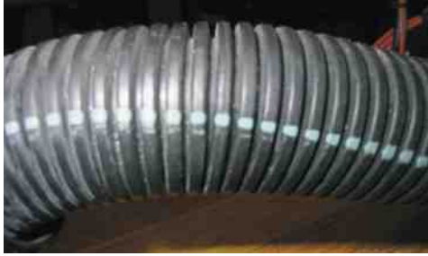
FIGURE 10-25 Conduit that has a paint strip is constructed of plastic that can withstand high underhood temperatures.
