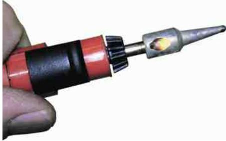
FIGURE 10-19 A butane-powered soldering tool. The cap has a built-in striker to light a converter in the tip of the tool. This handy soldering tool produces the equivalent of 60 watts of heat. It operates for about 1/2 hour on one charge from a commonly available butane refill dispenser.
