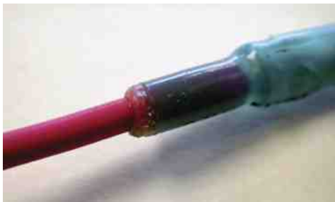
FIGURE 10-24 Heating the crimp-and-seal connector melts the glue and forms an effective seal against moisture.
