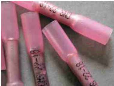
FIGURE 10-23 A typical crimp-and-seal connector. This type of connector is first lightly crimped to retain the ends of the wires and then it is heated. The tubing shrinks around the wire splice, and thermoplastic glue melts on the inside to provide an effective weather-resistant seal.
