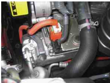
FIGURE 10-27 Always follow the vehicle manufacturer's instructions which include the use of lineman's (high-voltage) gloves if working on circuits that are covered in orange conduit.
