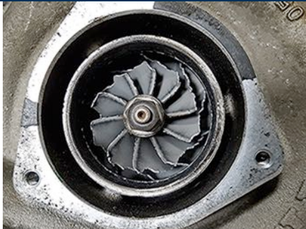
FIGURE 9–14 A turbocharger with damaged impeller blades. Small black plastic pieces were found around area indicating that air filter housing had been damaged when owner replaced air filter. Pieces from broken housing causes damage to turbocharger.
