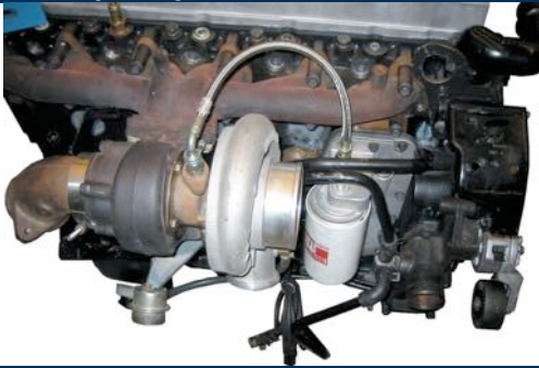
FIGURE 9-1 turbocharger on a Cummins inline six-cylinder diesel engine. Engine oil is fed to the center of the turbocharger to lubricate the bushings and returns to the oil pan through a return line.
