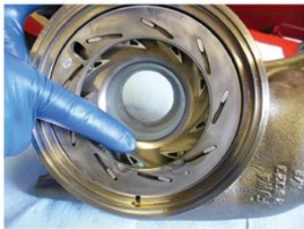
FIGURE 9-9 (a) the variable vane turbocharger from a Duramax diesel engine, showing the vanes in the extended position. This position creates a higher velocity exhaust stream being applied to the turbine blades when the engine speed is low.
