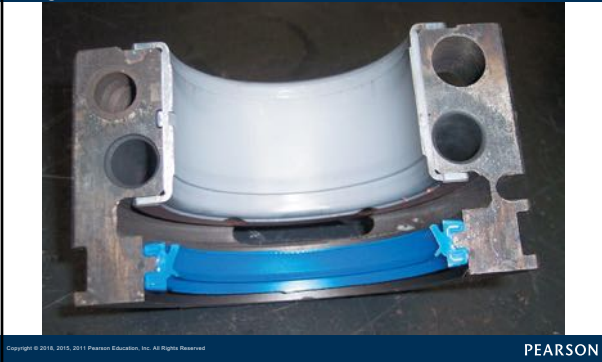
Figure 8-8 Lip-type rear main bearing seal in place in the rear main bearing cap. The lip should always be pointing toward the inside of the engine.
