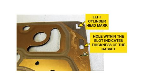
FIGURE 8–24 A head gasket from the left cylinder head on a Duramax V-8 diesel engine. The “L” means it is for the left head and the hole in the slot indicates its thickness.
