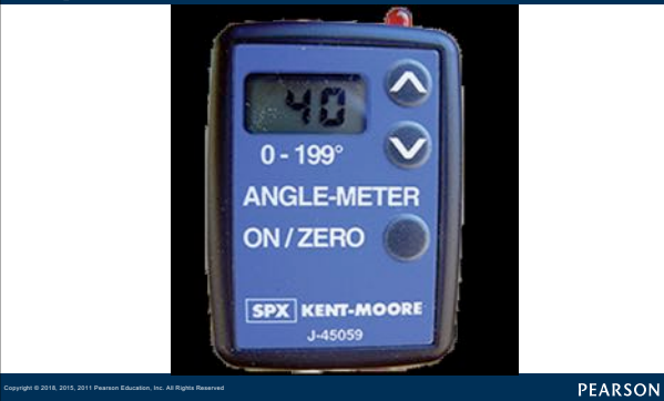
FIGURE 8-22 Torque angle can be measured using a special adaptor.
