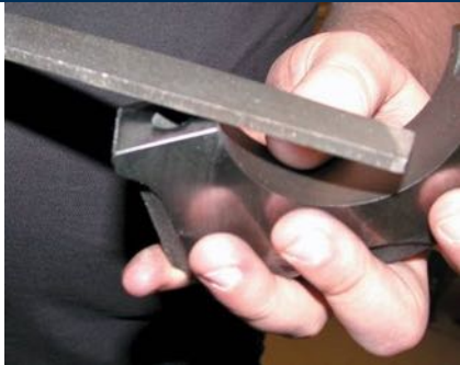
FIGURE 8–1 Deburring all sharp edges is an important step to achieve proper engine assembly.
