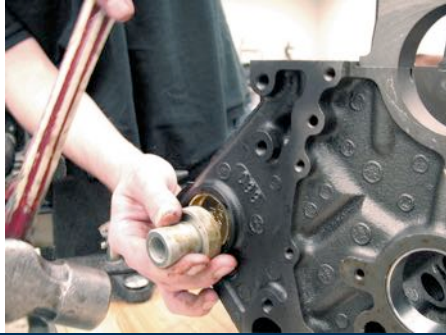
FIGURE 8-4 Sealer should be applied to the cup plug before being driven into the block
