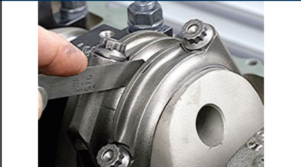
FIGURE 8-18 connecting rod side clearance is measured with a feeler gauge.
