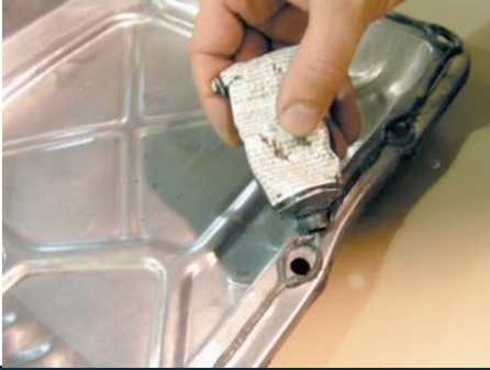
FIGURE 8-28 1/8 to 3/16 inch (3 to 5 mm) bead of RTV silicone on a parting surface with silicon going around the bolt hole..
