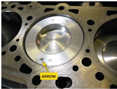
FIGURE 8-12 (B) Duramax diesel engine uses an arrow on the top of the piston to indicate the front of the engine.
