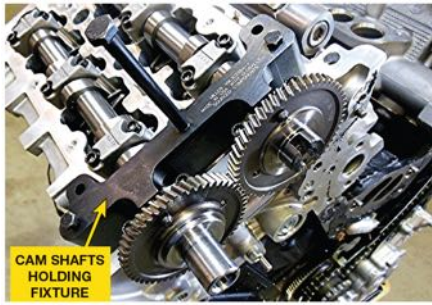
FIGURE 8–25 special holding fixture is required when installing the camshafts on the Fiat Chrysler 3.0 liter V-6 diesel engine to keep them aligned and in the proper position before the timing chain is installed
