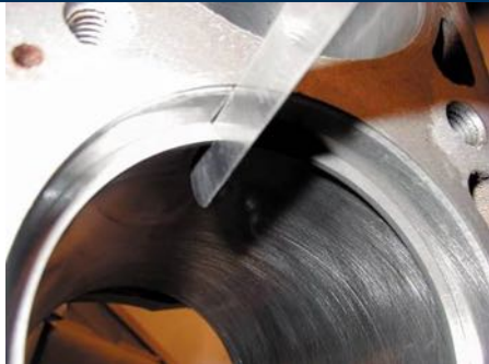
FIGURE 8-11 feeler gauge is used to check piston ring gap.
