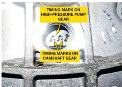
FIGURE 8–26 timing gears on Duramax diesel engine can be seen through an opening in timing cover for the high-pressure pump to camshaft. Duramax diesel HP Pump is timed so that fuel pressure regulator (FPR) solenoid commands at same time as piston strokes, which helps reduce vibration and noise.
