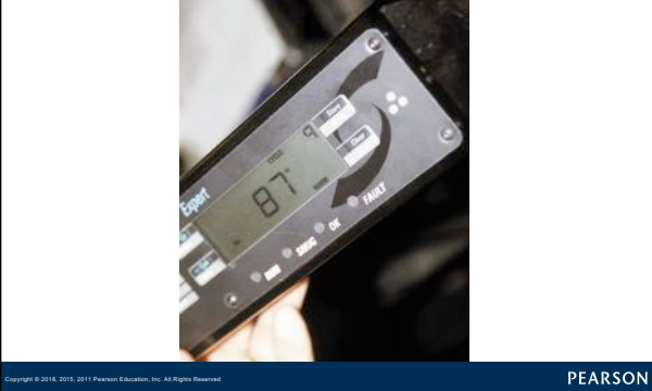
FIGURE 8–23 an electronic torque wrench showing number of degrees of rotation. These very accurate torque wrenches can be programmed to display torque or number of degrees of rotation.
