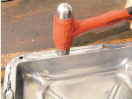
FIGURE 8–30 Using a hammer to straighten the gasket rail surface of the oil pan before installing a new gasket. When the retaining bolts are tightened, some distortion of sheet metal covers occurs. If the area around the bolt holes is not straightened, leaks can occur with the new gasket.
