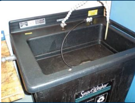
FIGURE 7-12 A microbial cleaning tank uses microbes to clean grease and oil from parts.
