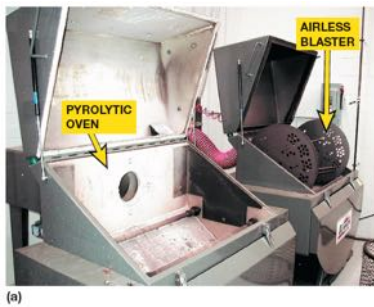
FIGURE 7-13 (a) A pyrolytic (high-temperature) oven cleans by baking engine parts. After parts have been cleaned, they are then placed into an airless blaster. This unit uses a paddle to scoop stainless steel shot from a reservoir and forces it against the engine part. The parts must be free of grease and oil to function correctly.
