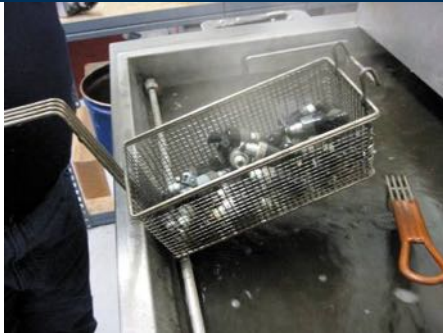
FIGURE 7-14 ultrasonic cleaner is used to clean fuel injectors.
