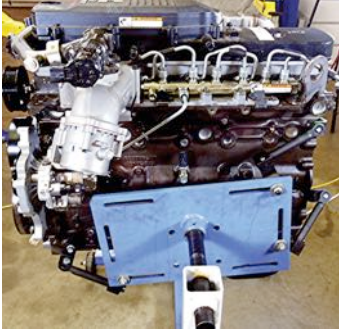
FIGURE 7-2 Cummins 6.7 liter inline six-cylinder diesel engine is so long that it is best to use an engine stand that supports the engine from the side rather than from the bell housing section of the block..
