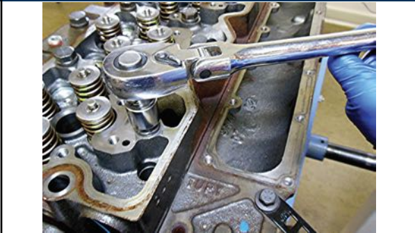
FIGURE 7-4 Cylinder head bolts being loosened on a Cummins 6.7-liter diesel engine, starting at the ends of the head and working toward the center.
