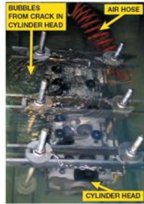
Figure 7-17 cylinder head is under water and being pressure tested using compressed air. Note that the air bubbles indicate a crack.
