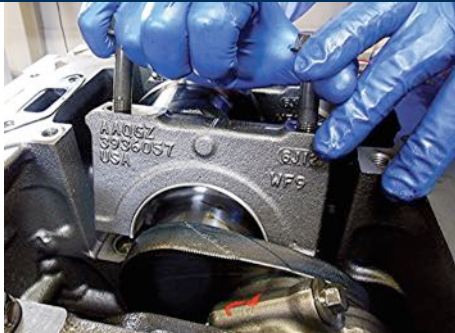
FIGURE 7-7 Main bearing cap being removed from a Cummins 6.7-liter diesel engine. The caps are marked so there was no need to mark their location or direction.
