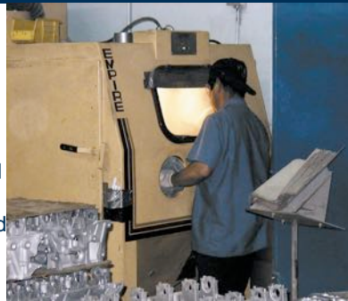
FIGURE 7-10 Smaller engine parts can be blasted clean in a sealed cabinet.
