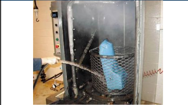
FIGURE 7–11 A pressure jet washer is similar to a large industrial-sized dishwasher. Each part is then rinsed with water to remove chemicals or debris that may remain there while it is still in the tank.
