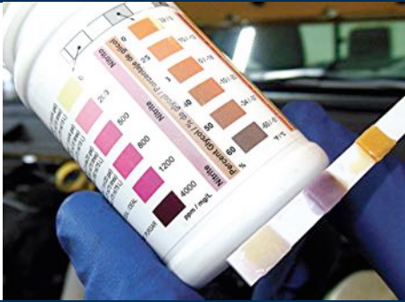
FIGURE 6-4 Coolant condition can be easily checked using test strips.
