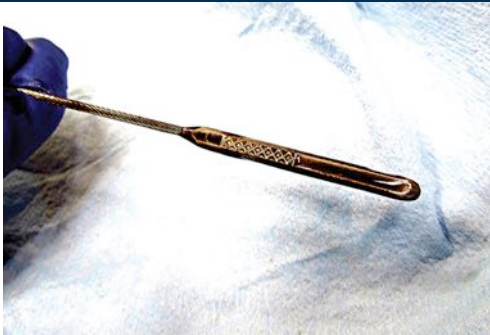
FIGURE 6-3 Checking engine oil level and condition is almost always first step in diagnosis of any diesel engine diagnosis.
