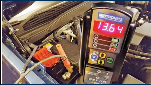
FIGURE 6-16 Midtronics tester that can not only test battery, but can also detect faults with starter & alternator.
