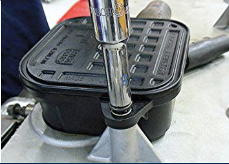
FIGURE 6-7 crankcase breather being removed from valve cover of a 6.7 liter Cummins diesel engine.
