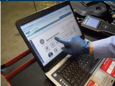
FIGURE 6-2 After checking for stored DTCs, wise technician checks service information for any technical service bulletins that may relate to the vehicle being serviced.
