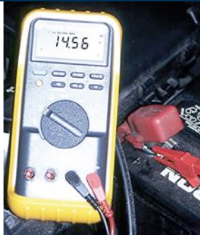
FIGURE 6–20 With engine running, the battery voltage should be between 13.5 and 15 volts.
