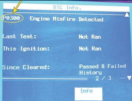
FIGURE 6-10 GM Tech 2 scan tool display showing a random misfire DTC (P0300) has been detected.
