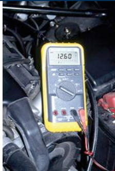
FIGURE 6-15 battery that measures 12.6 volts or higher after the surface charge has been removed is 100% charged.
