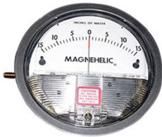
FIGURE 6-8 gauge measures low positive and negative pressures in units of inches of water. (1 inch of mercury (in. Hg) equals 14 inches of water so this unit is very small.) Connect gauge to source that can measure crankcase pressure, usually at oil dipstick tube.
