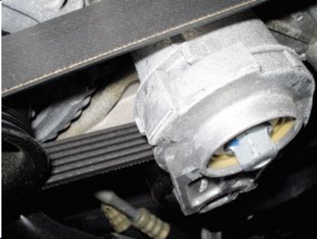
FIGURE 6-6 accessory belt tensioner. Most tensioners have a mark that indicates normal operating location. If belt has stretched, this indicator mark will be outside of normal range. Anything wrong with belt or tensioner can cause noise.
