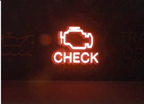
FIGURE 6-1 typical “Check Engine” light which should come on when ignition is first turned on as bulb check and then go out. If check engine light remains on, then PCM detected fault & DTC se
