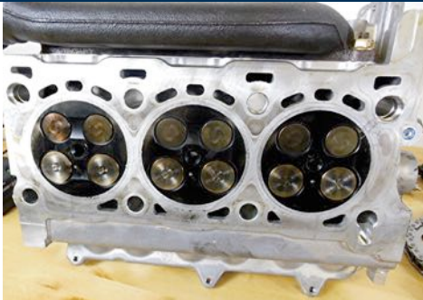
FIGURE 3-2 Four valve cylinder head from a Fiat Chrysler 3.0 liter diesel engine.
