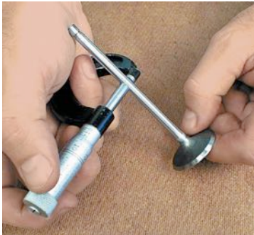
FIGURE 3–25 Diameter of the valve stem is being measured using a micrometer. The difference between the inside diameter of the valve guide and the diameter of the valve stem is the valve guide-to-stem clearance.
