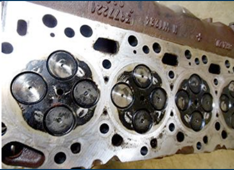
FIGURE 3-1(B) Cast iron Cummins 6.7 liter inline six cylinder diesel engine cylinder head.
