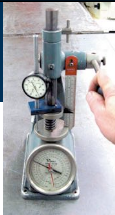
FIGURE 3–11 one popular type of valve spring tester used to measure compressed force of valve springs. Specifications usually include (1) free height (height without being compressed), (2) pressure at installed height with valve closed, and (3) pressure with valve open to height specified.
