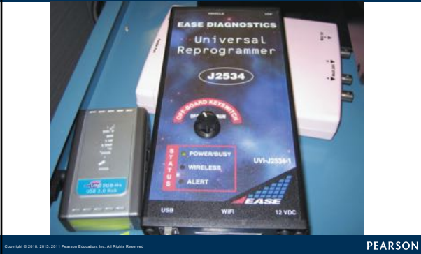
FIGURE 21-13 A typical J2534 universal reprogrammer that uses the J2534 standards.
