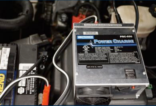
FIGURE 21–10 battery charger that does not introduce any alternating current (AC) when charging battery is extremely important when programming a PCM.
