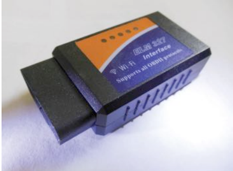
FIGURE 21-6 Bluetooth adapter that plugs into DLC and transmits global OBD-II information to a smart phone that has a scan tool app installed.
