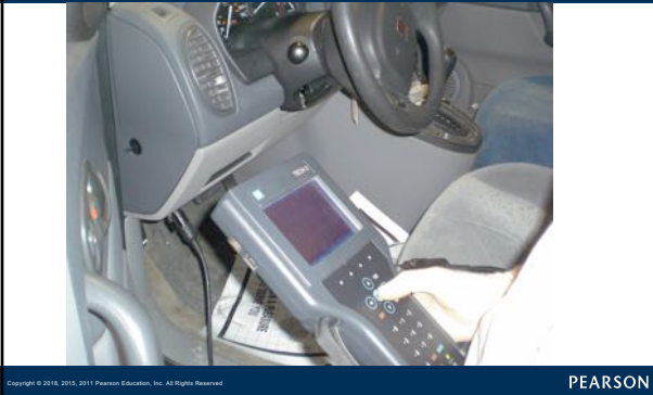
FIGURE 21-7 first step in reprogramming procedure is to determine current software installed, using a scan tool. Not all scan tools can be used. In most cases using factory scan tool is needed for reprogramming unless scan tool is equipped to handle reprogramming
