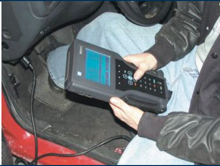
FIGURE 21-5 TECH 2 scan tool is factory scan tool used on General Motors vehicles.
