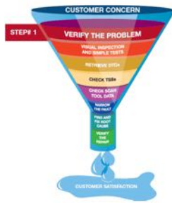
FIGURE 21–2 Step #1 is to verify customer concern or problem. If problem cannot be verified, then repair cannot be verified.
