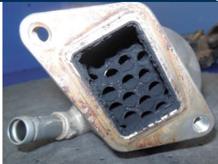
FIGURE 20-7 A partially clogged EGR cooler. While they may be able to be cleaned, most are simply replaced because the time needed to clean them exceeds the cost of a new part.
