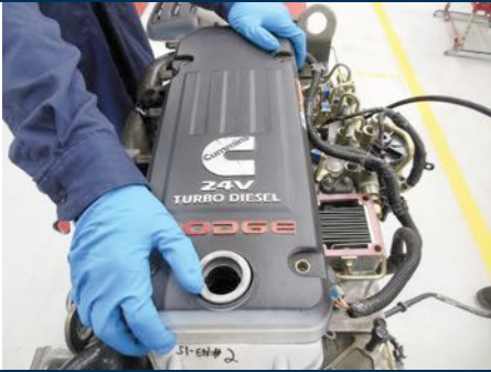
FIGURE 20-8 (a) To get access to crankcase breather filter, top plastic cover has to be removed from this Cummins 6.7 liter diesel engine.
