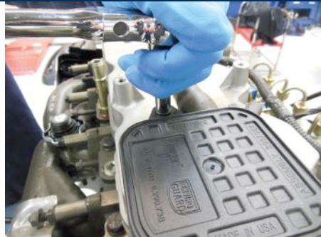
FIGURE 20-8 (b) crankcase breather filter is attached to cylinder head cover and can be replaced if needed based on reading from the crankcase pressure sensor.
