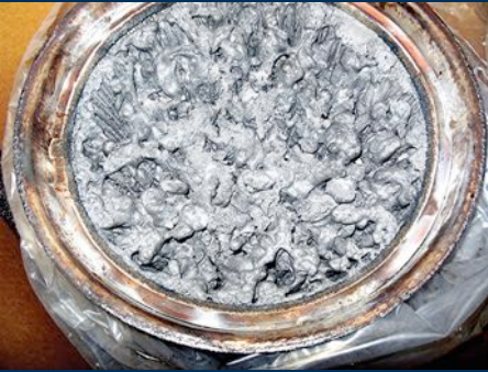
FIGURE 20-6 failed particulate filter that was so hot from being over-fueled it caused the substrate to melt.
