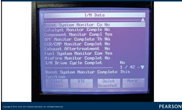
FIGURE 20-5 boost system monitor information as displayed on a Tech 2 scan tool used on Duramax diesel.
