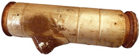
FIGURE 20-4 NOx absorber catalyst used by some OEMs usually before 2010 when NOx emission standards were greatly reduced, requiring most manufacturers to start using SCR
