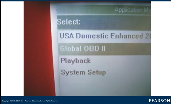
FIGURE 19-5 global OBD II can be accessed from the main menu on all factory-level aftermarket and some original equipment scan tools.
