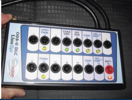
FIGURE 18-24 breakout box (BOB) used to access BUS terminals while using scan tool to activate modules. This breakout box is equipped with LEDs that light when circuits are active.
