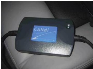
FIGURE 18–12 A CANdi module will flash green LED rapidly if communication is detected.
