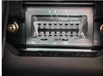
FIGURE 18–21 DLC from pre-CAN Acura. It shows terminals in cavities 4, 5 (grounds), 7, 10, 14, &16 (B+).
