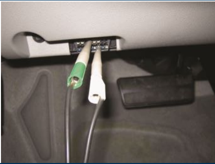
FIGURE 18-28 Use front-probe terminals to access DLC. Always follow specified back-probe & front-probe procedures as found in service information
