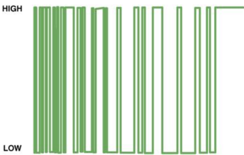
FIGURE 18.29 (a) Data is sent in packets, so it is normal to see activity then a flat line between messages
