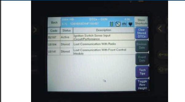
FIGURE 18–22 Honda scan display showing B and two U codes, all indicating a BUS-related problem(s)
