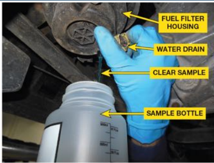
FIGURE 16-7 Many manufacturers recommend that the water be drained every 30 days. When all the water is drained, only diesel fuel will be coming out of the drain.
