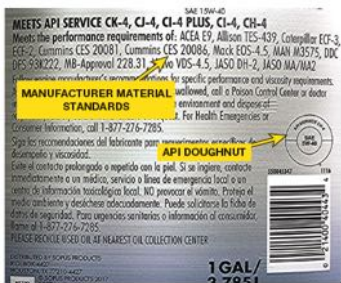
FIGURE 16-5 Diesel engines manufactured for use after January 1, 2017, may require the use of diesel motor oil that has a rating of CK-4.
