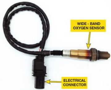
FIGURE 15–19 oxygen sensor is used to monitor operation of EGR system.
