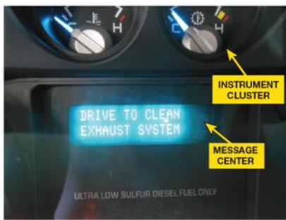
FIGURE 15–14 DPF warning lamp used to warn driver vehicle needs to be driven in manner that regeneration event can occur.
