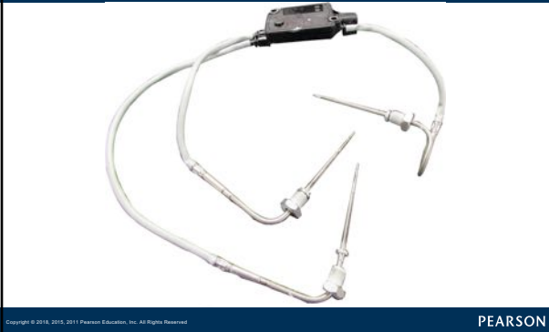
FIGURE 15–17 Temperature sensors are used by PCM to monitor function of various components in aftertreatment system.
