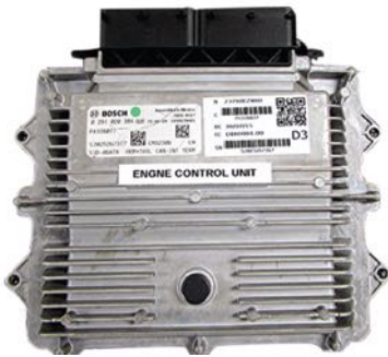
FIGURE 13–17 powertrain control module contains driver circuits and DC-DC converter needed to operate injectors.
