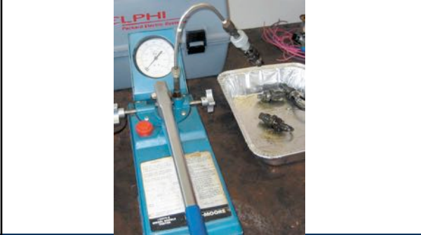
FIGURE 13–28 A typical pop tester used to check the spray pattern of a diesel engine injector.
