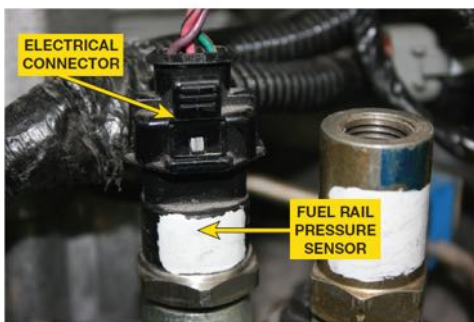
FIGURE 13-4 fuel rail pressure sensor provides feedback to the powertrain control module so the high-pressure fuel pump can operate most efficiently.
