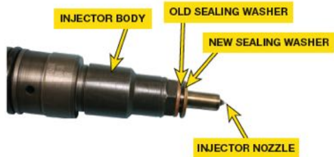
FIGURE 13–24 failure to install injector with its sealing washers properly can lead to leakage and system performance problems.
