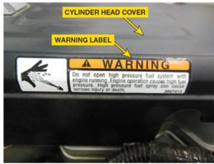
FIGURE 13-2 example of an under hood high-pressure fuel warning decal, warning of dangers related to system.
