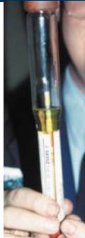
Figure 11-2 Testing the API viscosity of a diesel fuel sample using a hydrometer.
