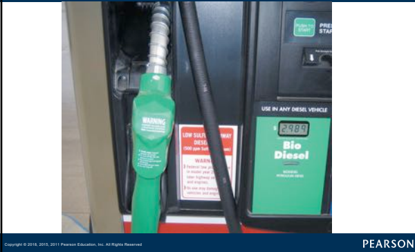
FIGURE 11-4 A pump decal indicating that the biodiesel fuel is ultra-low-sulfur diesel (ULSD) and must be used in 2007 and newer diesel vehicles.
