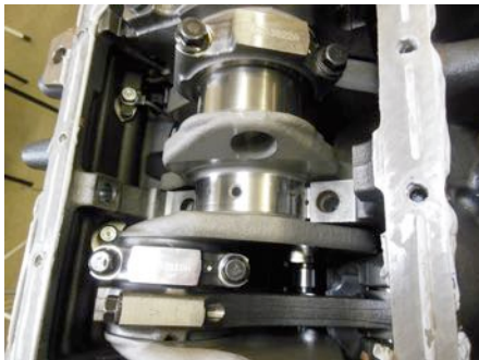
FIGURE 1-11 crankshaft determines the stroke of the engine, which is the difference between the centerline of the crankshaft journal and the centerline of the connecting rod journal
