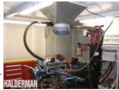
Gas Engine On Engine Dynamometer
