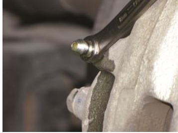
FIGURE 8.9 Gravity bleeding is simply opening the bleeder valve and allowing gravity to force the brake fluid out of the bleeder valve.
