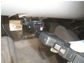
FIGURE 8.16 To perform an automated brake bleed procedure on an antilock brake system, first connect a factory or enhanced scan tool to the data link connector (DLC) located under the dash on this vehicle.
