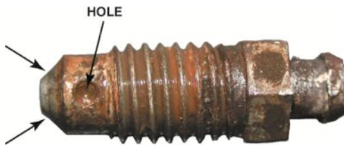
FIGURE 8.2 Typical bleeder valve from a disc brake caliper. The arrows point to the taper section that does the actual sealing. It is this taper that requires a shock to loosen.
