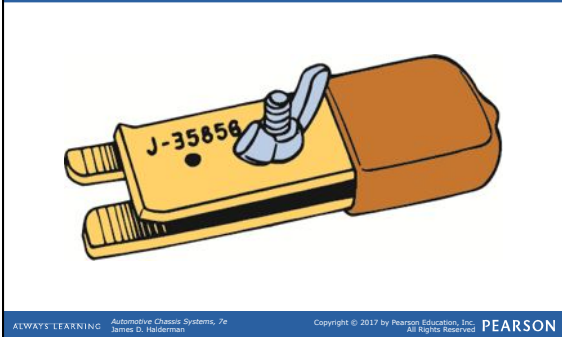
FIGURE 8.14 Special bleed valve tools are often required when bleeding some ABS units such as the Kelsey-Hayes 4WAL system.
