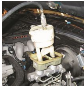
FIGURE 8.11 Brake fluid under pressure from the power bleeder is applied to the top of the master cylinder.
