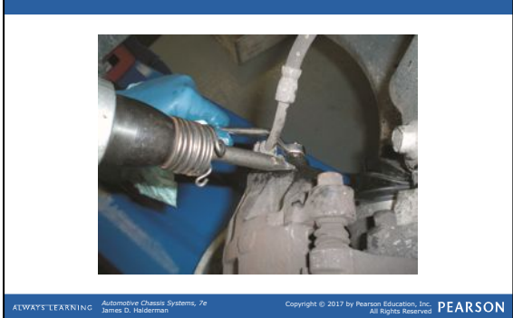
FIGURE 8.4 Using an air punch next to the bleeder valve to help "break the taper" on the bleeder valve.
