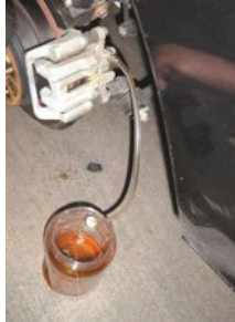
FIGURE 8.6 Bleeding brakes using clear plastic tubing makes it easy to see air bubbles.
