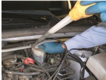
FIGURE 8.19 A turkey baster can be used to remove the old brake fluid from the master cylinder reservoir.
