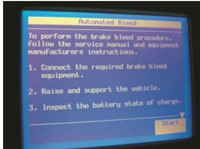
FIGURE 8.18 Scroll through the menus and select automated bleed procedure and follow the on-screen instructions.
