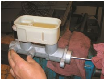
FIGURE 8.1 Bench bleeding a master cylinder. Always clamp a master cylinder in a vise by the mounting flange to prevent distortion of the cylinder bore.
